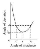
If the angle of incidence is increased gradually, then the angle of deviation first decreases, attains a minimum value  $(\delta_m)$ , and then again starts increasing. When angle of deviation is minimum, the prism is said to be placed in the minimum deviation position.
