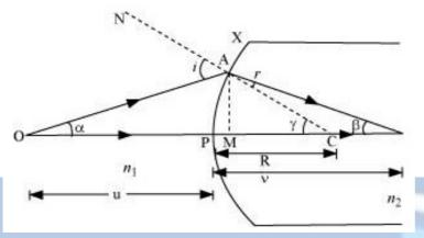
Let a spherical refracting surface XY separate a rarer medium of refractive index  $n_1$  from a denser medium of refractive index  $n_2$ . Let P be the pole, C be the centre and
