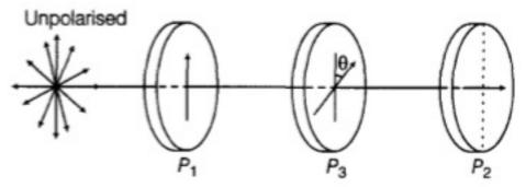
Let  $I_0$  be the intensity of polarised light after passing through the first polariser  $P_1$ . If  $\theta$  is the angle between the axes of  $P_1$  and  $P_3$ , then the intensity of the polarised light after passing through  $P_3$  will be  $I = I_0 \cos^2 \theta$ . As,  $P_1$  and  $P_2$  are crossed, the angle between the axes of  $P_1$  and  $P_2$  becomes 90°.
