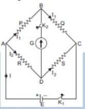
A battery is connected across A and C, while a galvanometer is connected B and D. Current is absent in the galvanometer's balance point.
