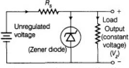
Excess current bypass when  $V_{ext} \ge V_{z}$
