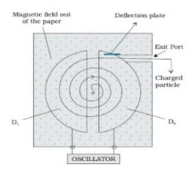
Working Principle: The cyclotron uses crossed electric and magnetic fields which increases the kinetic energy of a charged particle without changing its frequency of revolution.
