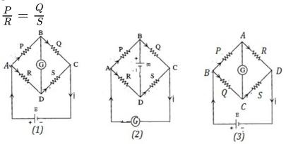
When the battery and the galvanometer are interchanged, the circuit takes the form (2). The circuit (2) can be re drawn as circuit (3). The ratio of the resistances in the bridge balanced condition is  $\frac{P}{Q} = \frac{R}{S}$  which is same as,  $\frac{P}{R} = \frac{Q}{S}$
