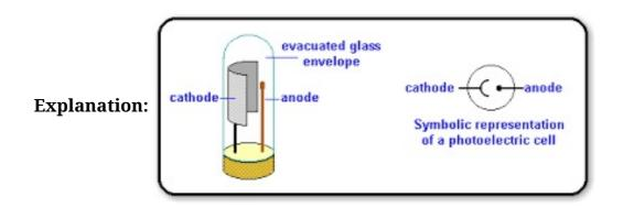
A photo cell is a device which converts light energy into electric energy.
