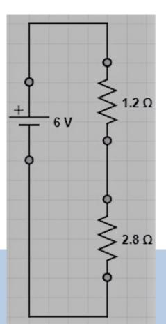
Total resistance of the circuit = 1.2+ 2.8 =  $4\Omega$  [:: these two are connected in series combination] Net current drawn from the cell,
