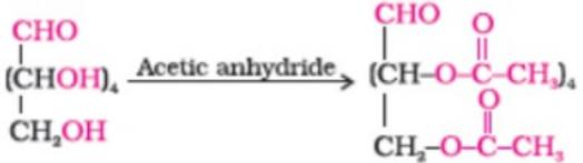
iii. Chemical reaction to show that open structure of D-glucose contains the aldehyde as carbonyl group:
