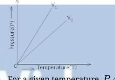
For a given temperature,  $P \propto \frac{1}{V}$  therefore when the gas is heated in a small vessel (Volume V<sub>1</sub>), the pressure will increases more rapidly than when heated in a large vessel (Volume V<sub>2</sub>). As a result, the slope of P - T graph will be more in case of small vessel than that of large vessel.
