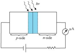
When visible light of energy ( $hv > E_g$ ) enters its depletion region, the electron-hole pairs are generated. These charge carriers are separated by the junction's electric field and are made to flow across the junction and cause reverse saturation current.
