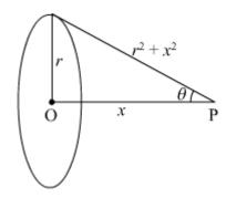
We need to find the electric field due to this charged ring at a point on the axis of the ring at a distance x from its centre.
