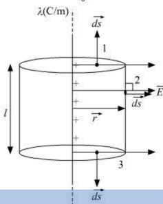
In the diagram we have taken a cylindrical gaussian surface of radius = r and length = l.
