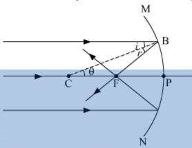
Consider a ray of light AB, parallel to the principal axis and incident on a spherical mirror at point B. The normal to the surface at point B is CB and CP = CB = R is the radius of curvature. The ray AB, after reflection from a mirror, will pass through F (concave mirror) or will appear to diverge from F (convex mirror) and obeys the law of reflection i.e. i = r.
