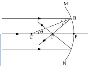
Consider a ray of light AB, parallel to the principal axis and incident on a spherical mirror at point B. The normal to the surface at point B is CB and CP = CB = R is the radius of curvature. The ray AB, after reflection from a mirror, will pass through F (concave mirror) or will appear to diverge from F (convex mirror) and obeys the law of reflection i.e. i = r.
