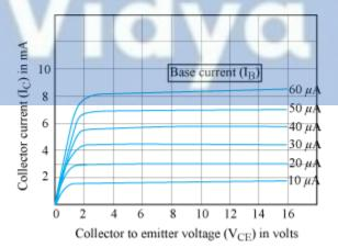
The output characteristics describe the relationship between output current ( $I_C$ ) and output voltage ( $V_{CE}$ ).
