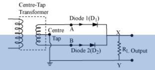
When the voltage at A with respect to the center tap is positive, and the voltage at B is negative. Then,  $D_1$  is forward biased and  $D_2$  is reversed biased. Hence,  $D_1$  conducts and  $D_2$  does not.
