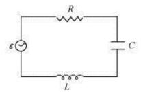
An ac source E having a voltage of  $v = v_m \sin \omega t$  is applied across the given LCR circuit.
