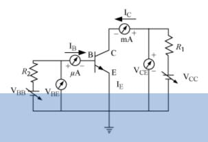
Variation of collector current  $I_C$  with the collector – Emitter voltage  $V_{CE}$  is called output characteristics
