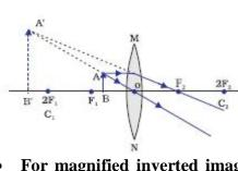
For magnified inverted image – object between F and 2F of a convex lens
