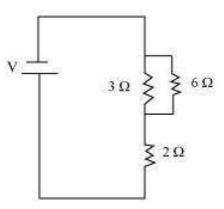
Since, 3  $\Omega$  and 6  $\Omega$  resistors in parallel, so the net resistance
