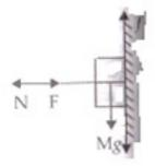
F = N And f = Mg  $\Rightarrow \mu F = Mg$ or  $F = \frac{Mg}{\mu}$  is the minimum force to hold the block against the wall at rest.
