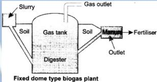
The biogas plant has a dome-like structure built with bricks. A slurry of cow-dung and water is made in the mixing tank from where it is fed into the digester. The digester is a sealed chamber in which there is no oxygen.
