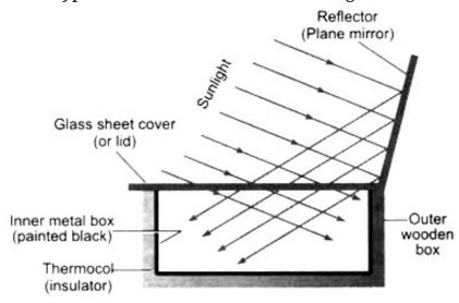
Construction of a box-type solar cooker:
