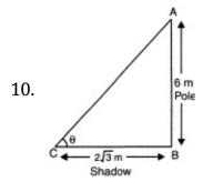
Let the Sun's elevation be  $\theta$ Length of pole = 6 m, length of shadow =  $2\sqrt{3}$ m From  $\triangle ABC$ ,  $\frac{AB}{BC} = \tan \theta$ ( using Pythagoras theorem)  $\Rightarrow \quad \frac{6}{2\sqrt{3}} = \tan \theta$   $\Rightarrow \quad \tan \theta = \frac{3}{\sqrt{3}} = \sqrt{3} = \tan 60^{\circ}$  $\Rightarrow \quad \theta = 60^{\circ}$
