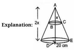
Radius of the cone = 20 cm Let the height of the cone be = 2x cm  $\Rightarrow$  The height of the smaller cone = x cm
